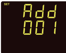
Fig 3-15 Communication Address Setup
