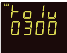
Fig 3-29 RO1 Alarm Threshold Range Setting
