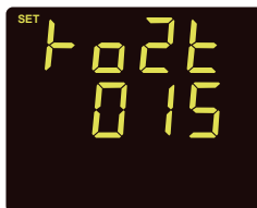
Fig 3-36 RO2 Alarm Delay Setting
