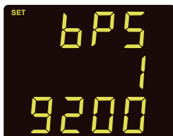
Fig 3-16 Baud Rate Setting
