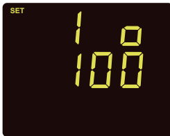
Fig 3-3 Full range shunt setting
