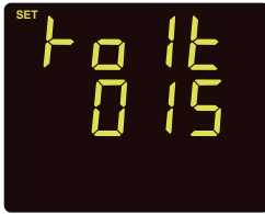
Fig 3-30 RO1 Alarm Delay Setting
