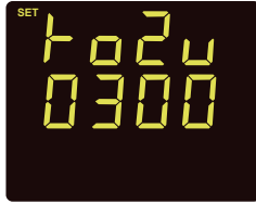
Fig 3-35 RO2 Alarm Threshold Range Setting
